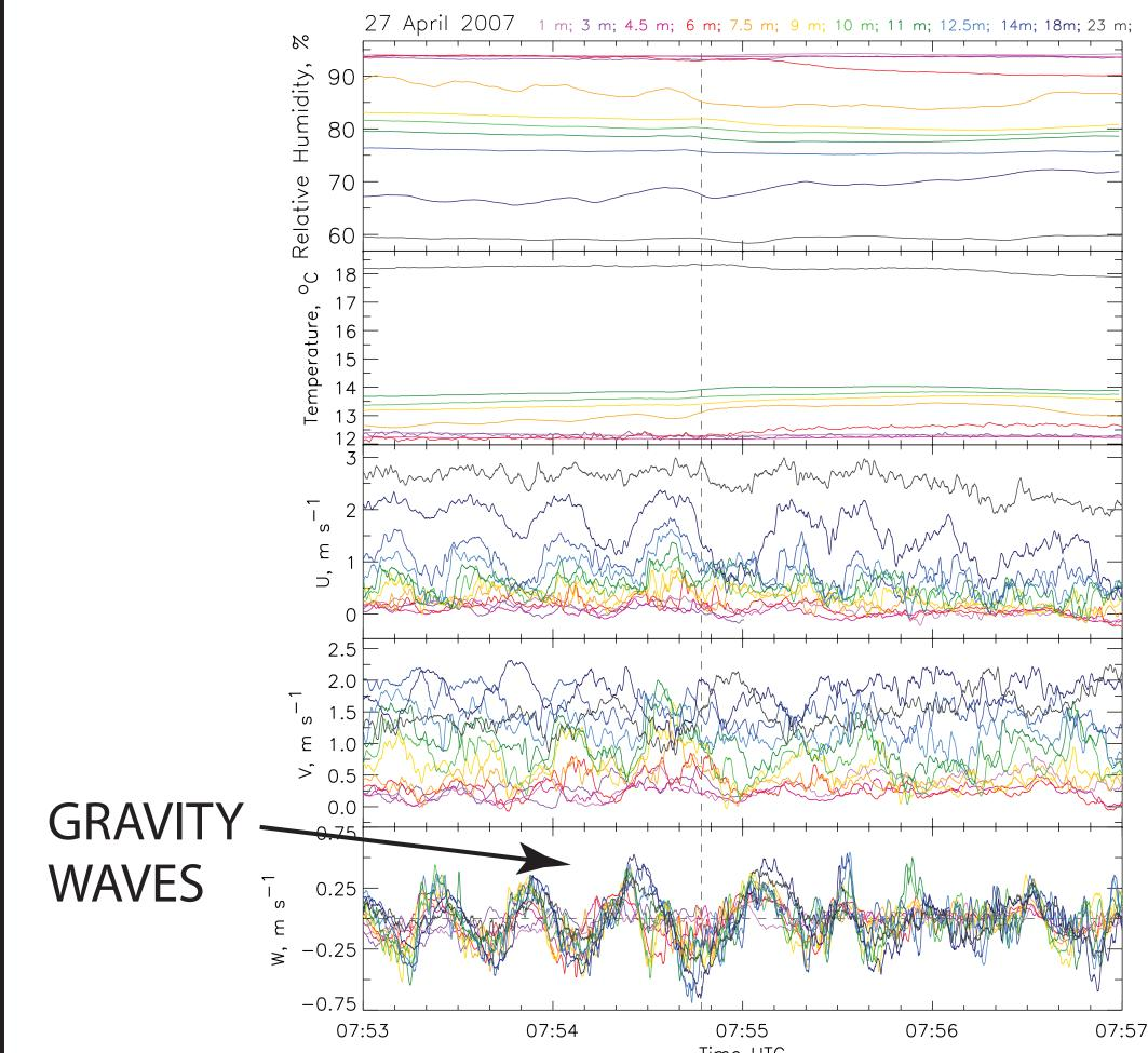
Above: Time-series data from multiple altitudes on the tower. The vertical velocity (bottom trace) shows the period of the waves in this case to be  $T_{\tau} \approx 38$  s. By combining lidar wavelength and tower period we determine that the phase speed of the waves in this case  $v = \lambda/T \approx 1.8$  m/s.
