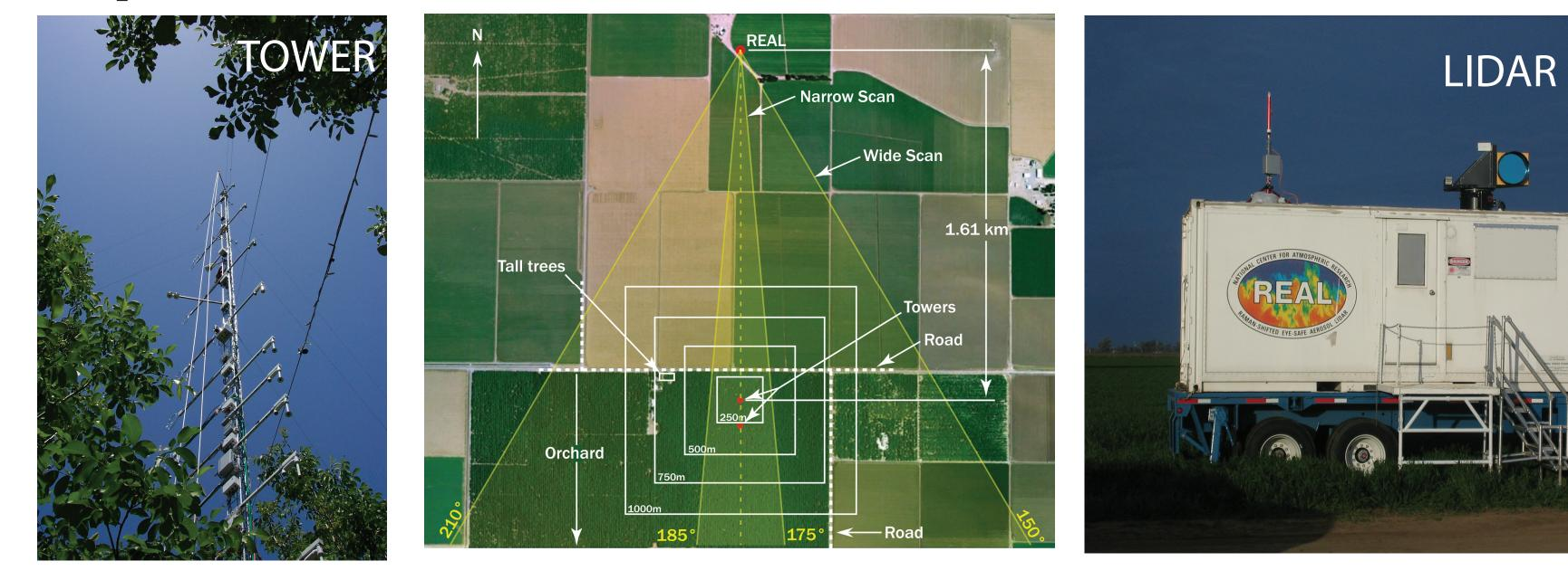
Sonic anemometers on the tower (left) sample 3-component wind velocities at 60 Hz. The lidar (right) scans over the orchard and through the tower at about 18 m altitude. Time-series data from the anemometers can be used to determine the period of the waves. Lidar scan images can be used to determine the wavelength of the waves. If the lidar scan images are collected rapidly enough, phase velocity can also be measured.
